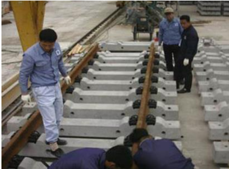
Figure 1.12. Prestressed concrete sleepers
