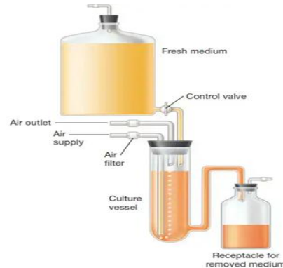
Figure 3. A continuous culture system: The chemostat
