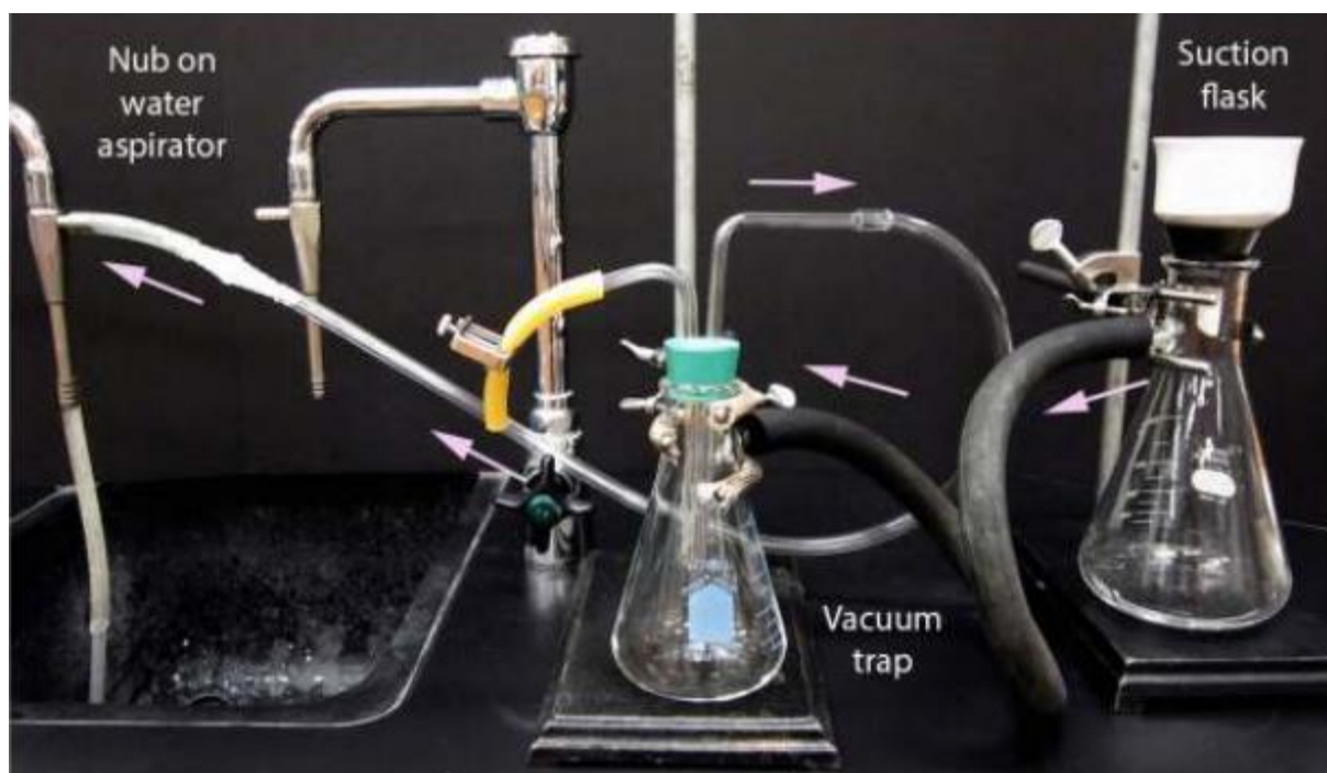
Figure 5 : Suction filtration flask attached to a vacuum trap and water aspirator.
