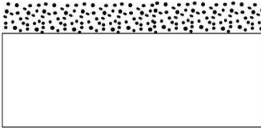
Fig.4. General corrosion affecting the surface of a metal
