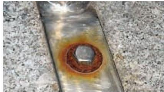
Fig.5. The puck is the element that exhibits the lowest resistance to corrosion.
