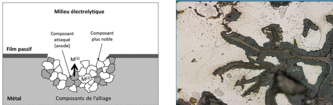
Fig.13. Selective Corrosion on cast iron
